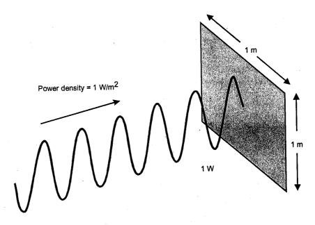
Electromagnetic wave passing through 1  $\text{m}^2$ . If the power passing through the area is 1 W, the wave has a power density of 1  $\text{W/m}^2$
